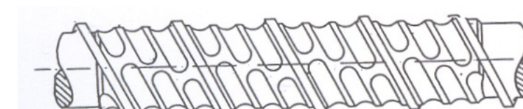
STRATA screw (little breakage, reorientation)
